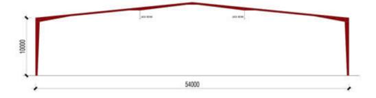
CÔNG TRÌNH: NHÀ XƯÔNG HÀI MỸ HẠNG MỤC: XƯÔNG SX CHỦ ĐẦU TƯ: CÔNG TY TNHH SX, TM HÀI MỸ ĐỊA ĐIỂM: ĐẶC ĐIỂM CÔNG TRÌNH: KÍCH THƯỘC 20 x 100M CAO: 4.5M, LẤP DỰNG Ở TỔNG 3 GIẢI PHÁP KẾT CẤU: CỘT BT, DÀN VÌ KĖO THẾP KHỐI LƯƠNG KẾT CẤU: 9.7 (KG/M2)
